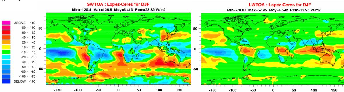
Figure 3: Comparison of the new scheme with CERES climatology for SW and LW net radiation at TOA with ARPEGE at operational resolution (T358C2.4) on DJF.
