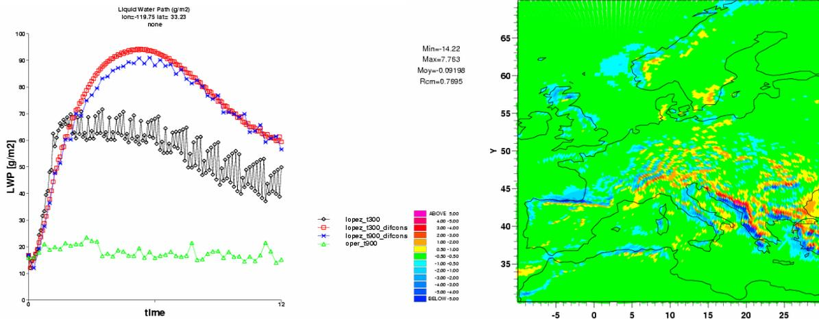
Figure 2a (left): Temporal evolution on 12 hours of Liquid Water Path (g/m<sup>2</sup>) on Eurocs stratocumulus case with the operational scheme ( $\Delta t=900s$ ) and the Lopez's scheme for 2 different time steps ( $\Delta t=300s$  and  $\Delta t=900s$ ) and with and without diffusion of conservative variables ("difcons").
